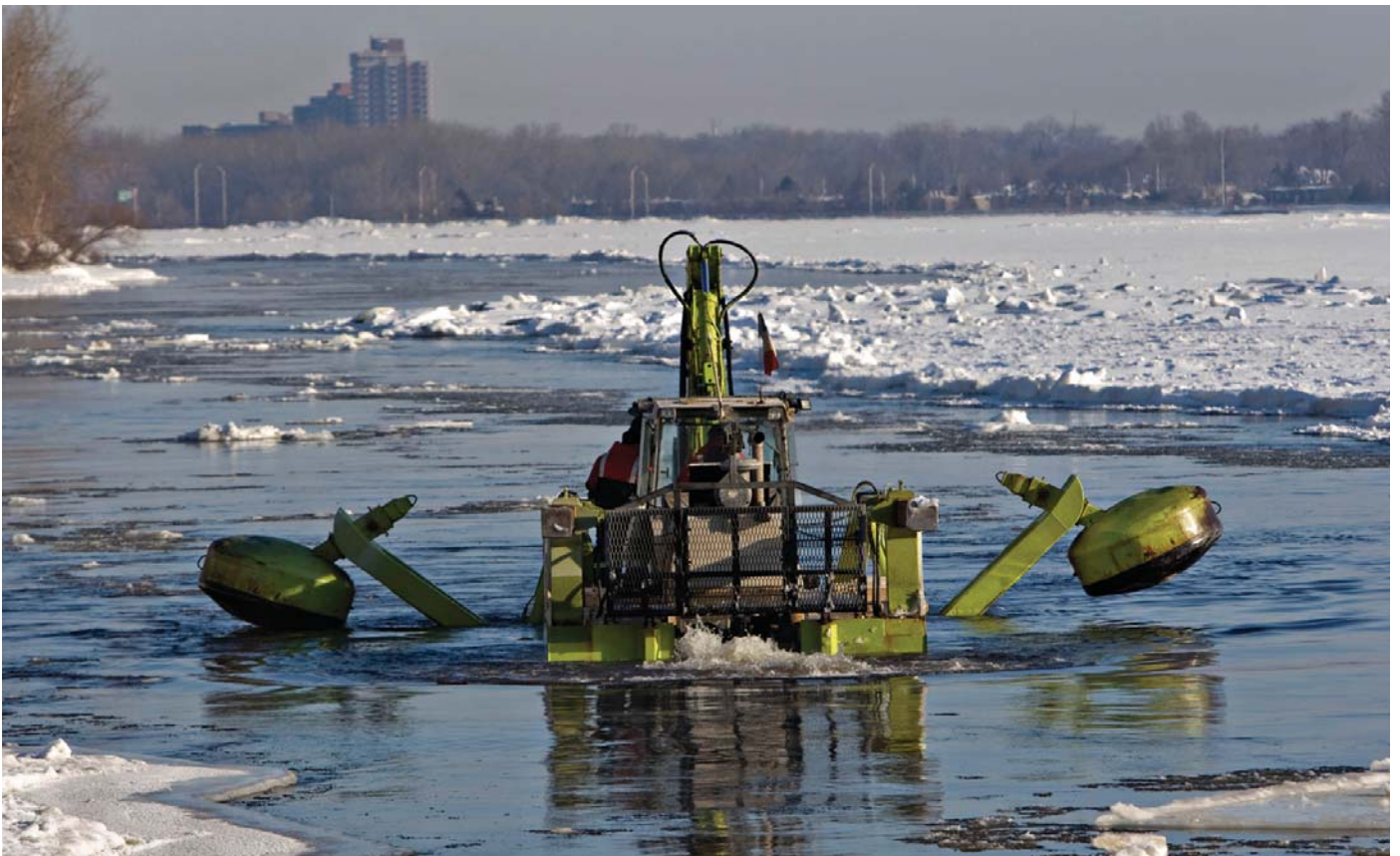
The Amphibex machine breaks up ice in Rivière des Prairies. (27/01/2009) Credit: © Ivanoh Demers, La Presse
