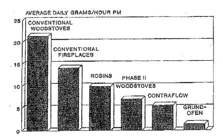
Masonry heater values normalized to a 1.0 kg/hr burn tale, the Phase II woodslove field evertes.
