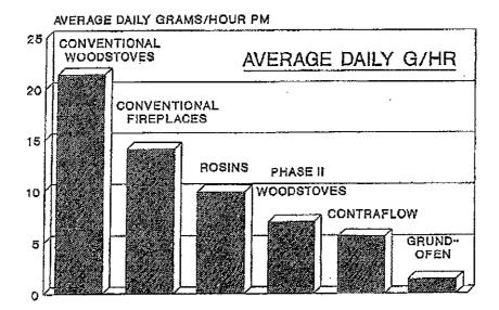
Masonry heater values normalized to a 1.0 kg/hr burn rate, the Phase II woodstove field average.
