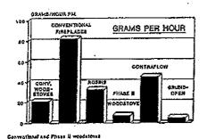
Figure 2. Comparison of PM grams per hour for woodstoves, fireplaces and masonry heaters.
