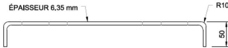
**PLATE-FORME - ÉLÉVATION**
