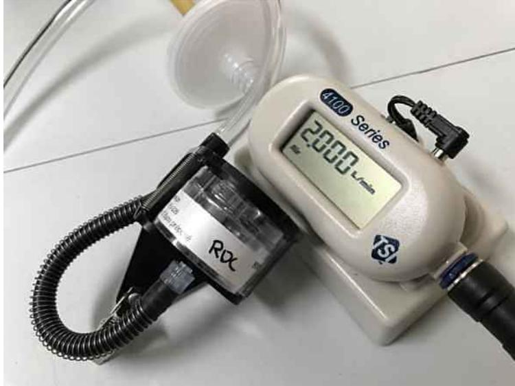
*CALIBRATION CONFORME – PRÉLÈVEMENT D'AIR POUR LE PLOMB*
