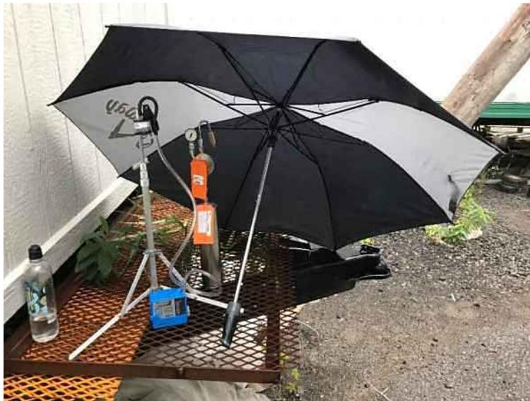
*PRÉLÈVEMENT D'AIR EXTÉRIEUR – NIVEAU REZ-DE-CHAUSSÉE – COV ET PLOMB*
