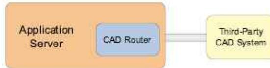
The CAD Router process residing on each Application Server operates redundantly (one is master, the other on standby), and is responsible for generating the CAD output and populating the Power 9-1-1 Lists Module's optional Abandoned Calls list.
