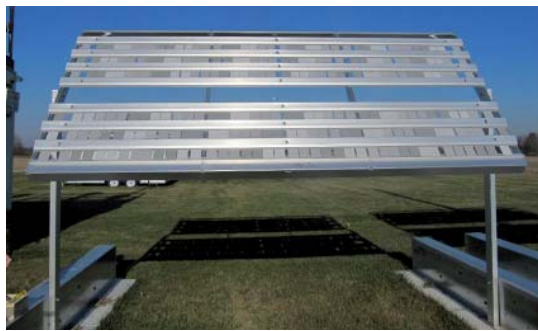
Sainte-Anne-de-Bellevue test bench with witness plates Photo credit: IREQ (Hydro-Québec), 2012
