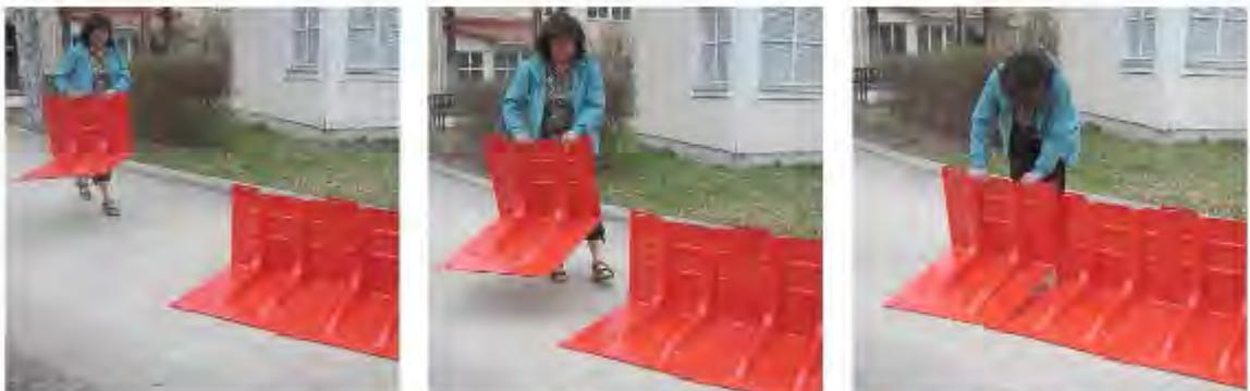
The boxes are easy to handle and move, and you can also adjust the setting of a constructed boxwall as long as the water has not started to press firmly against the base. But you must avoid dragging the boxes on the ground, as the sealing strips on the underside are vulnerable to wear.
