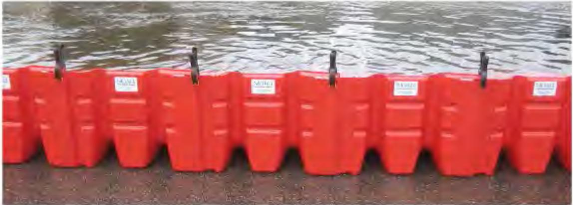
A NOAQ Boxwall is a mobile self-anchoring flood barrier. The NOAQ Boxwall BW50 creates a dam for water up to a height of 50 cm. The boxwall is so light that it can quickly be set up to protect buildings and other property against water damage, and also to keep roads open. A boxwall is designed for use on an even, firm surface, such as a paved street or a concrete floor. The boxwall is patented in a large number of countries.
