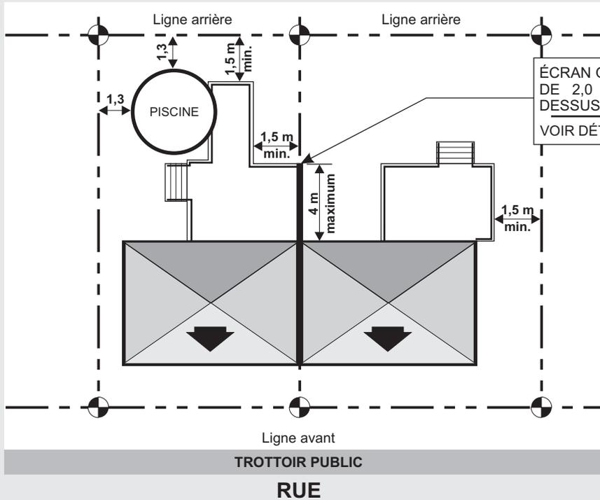
ÉCRAN OU TREILLIS D'UNE HAUTEUR DE 2,0 m DOIT ÊTRE ÉRIGÉ AU-DESSUS DU PLANCHER DU BALCON.
