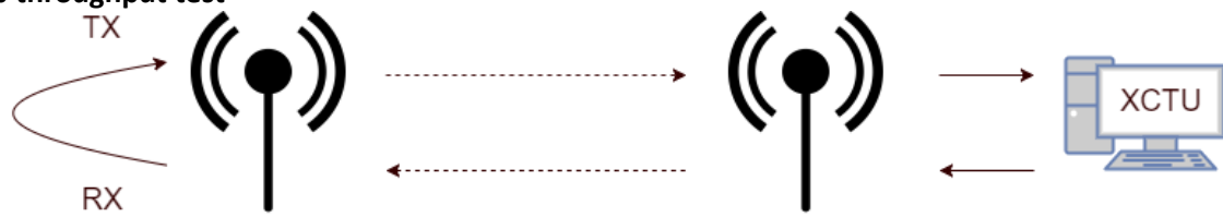
Figure 3.19: Zigbee throughput test setup.
