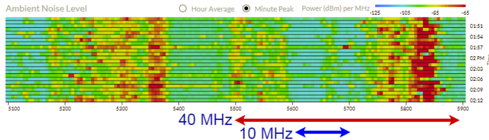
Figure 3.16: Spectrum analysis from Ubiquiti web GUI from an installed device in downtown Montreal.
