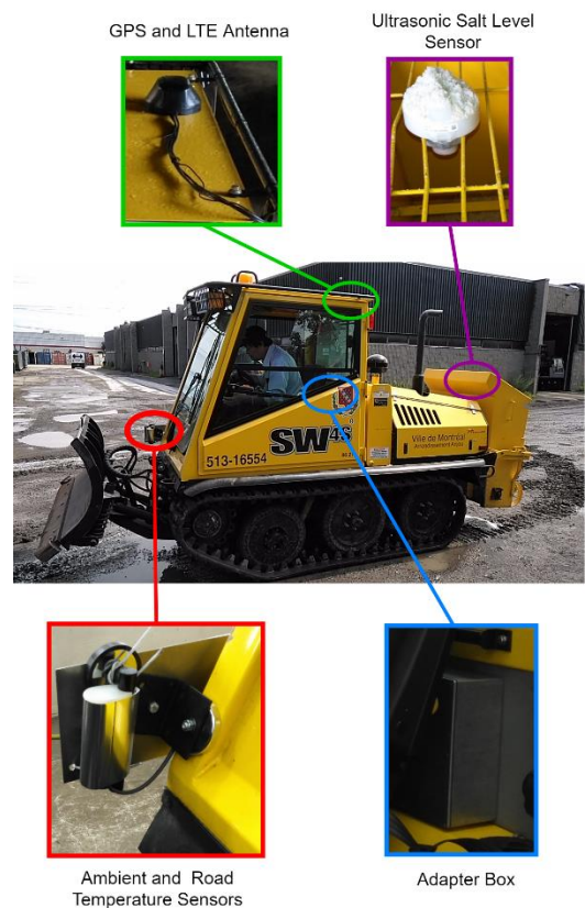
Figure 3.7: Installations of devices on the salt truck.
