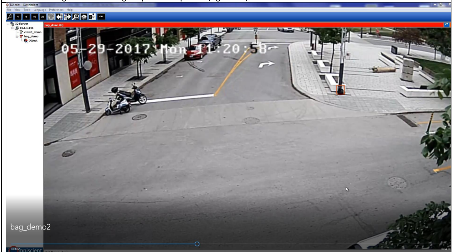
Unattended bag detection – bag drop-off without person (~ 25 seconds after person left the bag alone)
