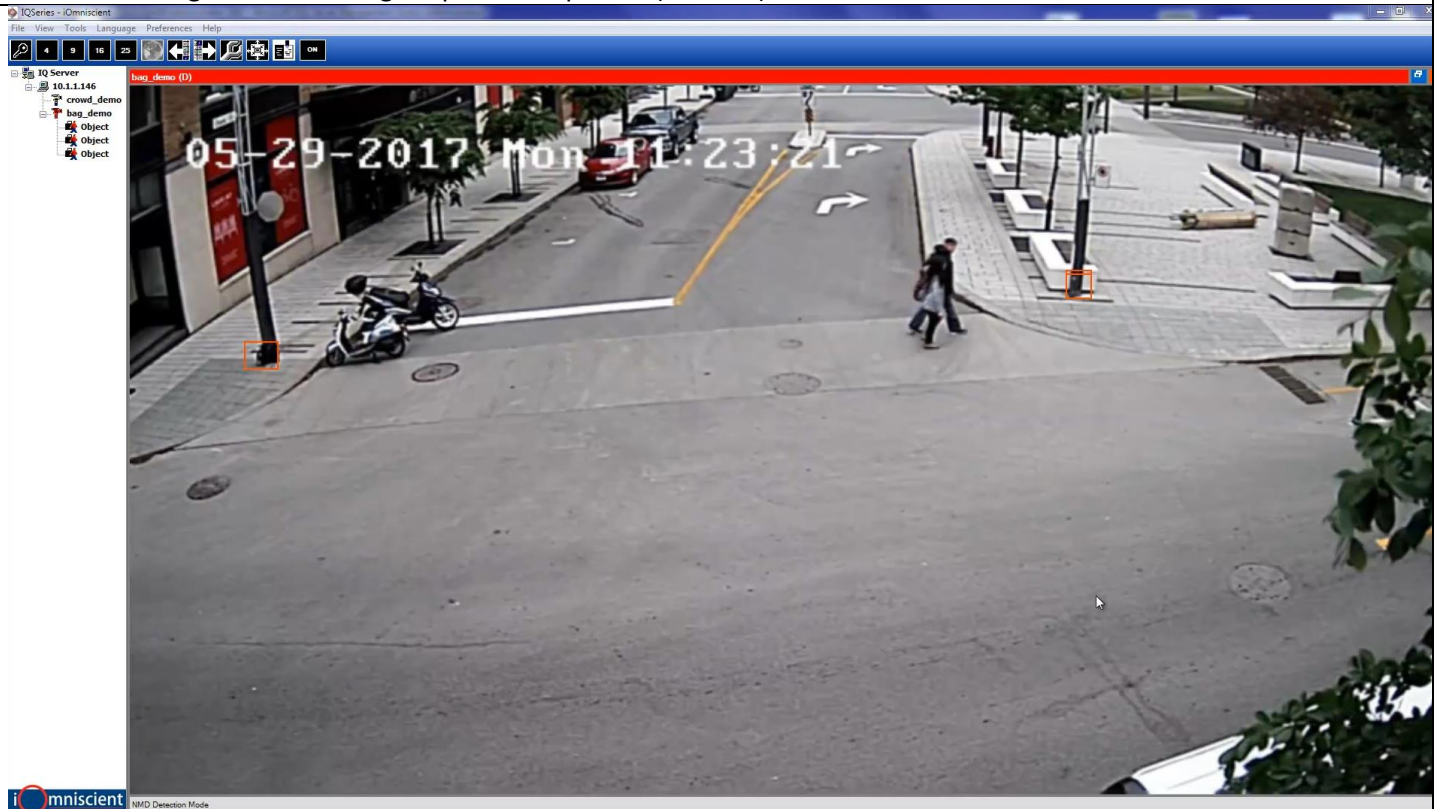
Unattended bag detection – bag drop-off without person – left side (~ 45 seconds after person left the bag alone)
