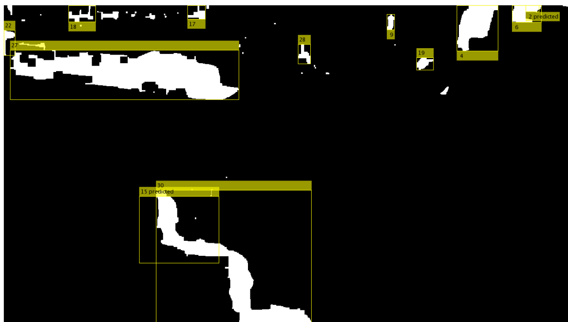
Figure 74: Moving object detection in the reference software after morphological operations
