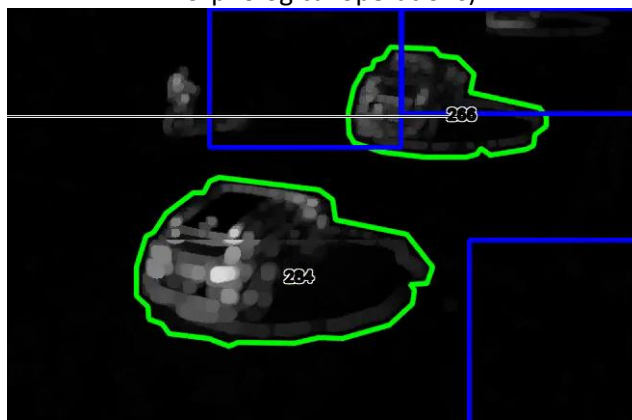
Figure 31: Initial difference frame (before application of shadow mask)
