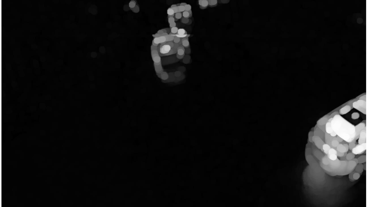
Figure 33: Difference frame after dilation operation
