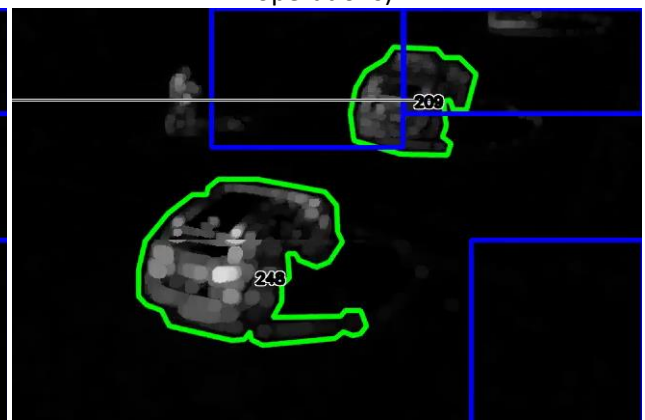
Figure 32: Final difference frame (after application of shadow mask)
