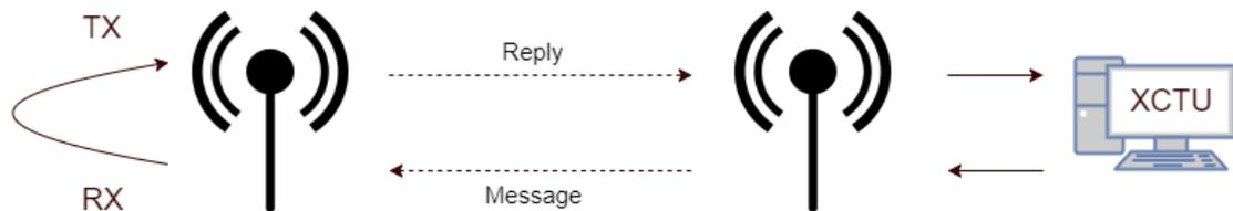
Figure 18: Diagram showing ZigBee throughput test setup
