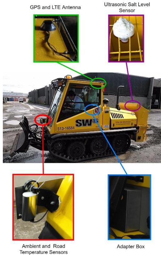
Figure 6: Pictures presenting mounted sensor installation locations on LTE-connected truck
