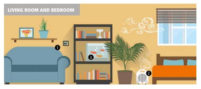
In living rooms and bedrooms, closets and cabinets are often built against an outdoor wall. The accumulation of clothes and belongings in these areas, combined with a lack of ventilation, can pose a risk of condensation, resulting in the proliferation of mould.
