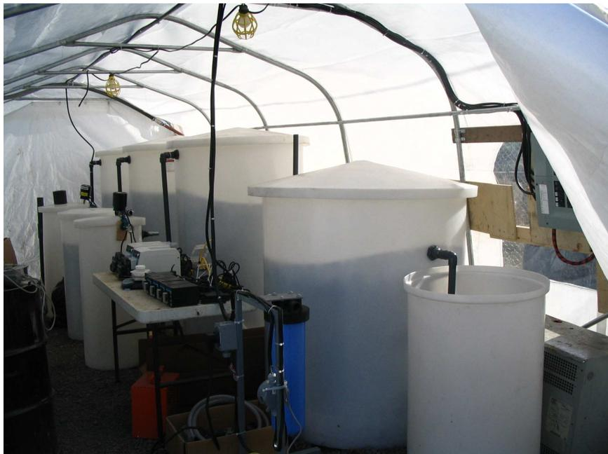
PHOTO 4: VUE DU MONTAGE DES ESSAIS PILOTES POUR LE SYSTÈME DE TRAITEMENT *MULTI-POINTS*
