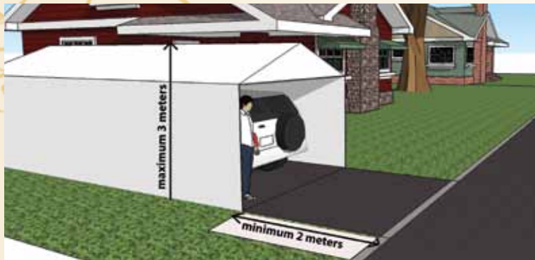
Minimum distance between the shelter and the curb
