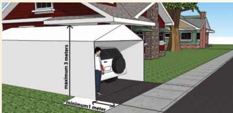
minimum distance between the shelter and the sidewalk
