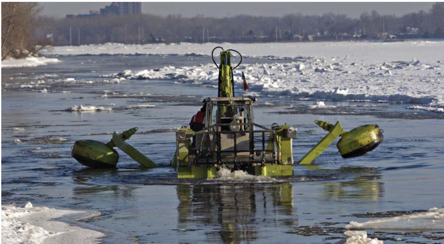
The froglike amphibious backhoe at work in the Des Prairies River. (27.01.2009) Credit: © Ivanoh Demers, La Presse
