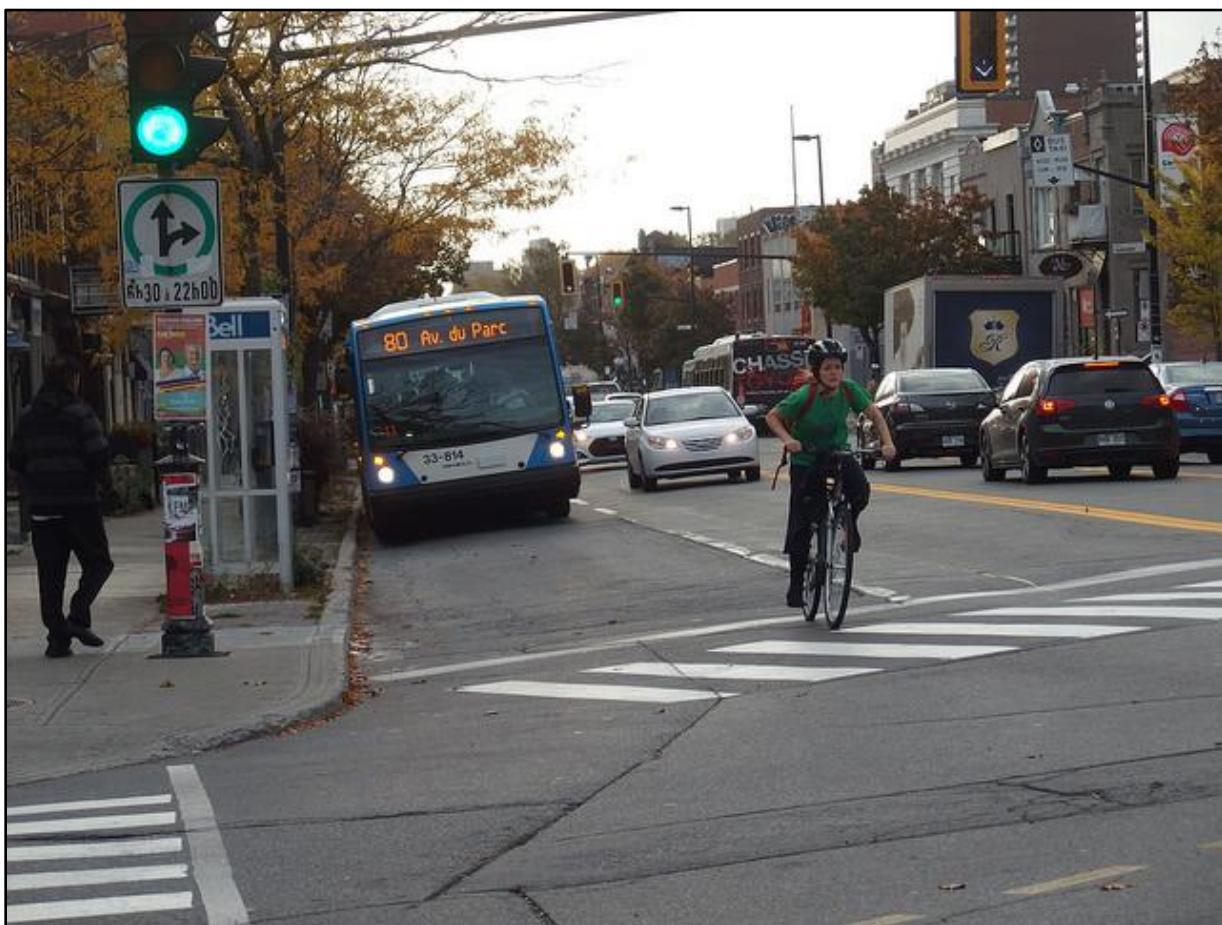
Image 8 Avenue du Parc – both buses and cyclists need a protected right-of-way in this high volume corridor. On-street parking is hindering such efforts.
