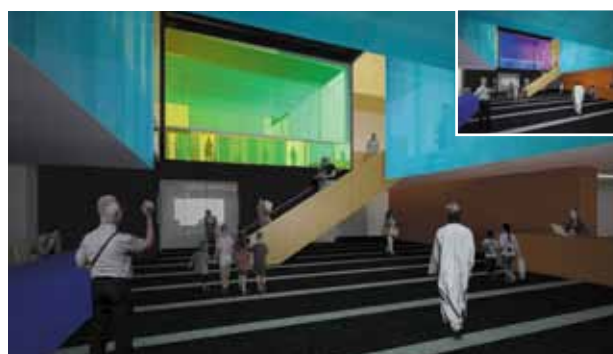
Constructed of tempered dichroic glass, the piece breaks down the light and shifts colour as the ambient daylight changes. With artificial lighting at night, the glass acts as a mirror.
